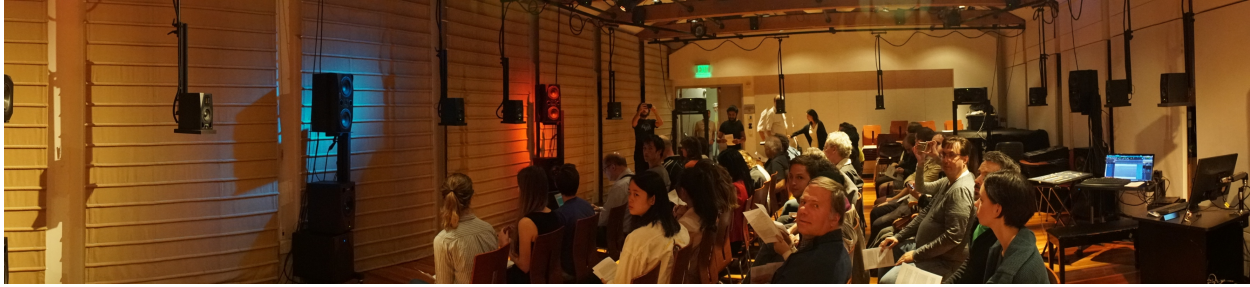
Figure 2: The Stage at CCRMA. This is a permanent installation of 56 full-range loudspeakers.
