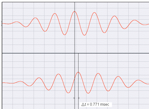
Figure 4: Ear signals after band-pass filtering, with fine time scale.
